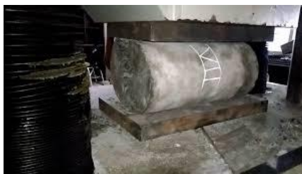
Gambar 4. Kuat tarik belah beton Sumber: https://youtube.com/watch?v=GiSgatiG7c
